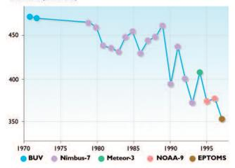
**Fig. 15.9.** Average total ozone over the Arctic (63° to 90° N) in March. 1971 and 1972 data are from the BUV instrument on the Nimbus-4 satellite; 1979–1993 data are from the Total Ozone Mapping Spectrometer (TOMS) on Nimbus-7; 1994 data are from the TOMS on Meteor-3; 1996 data are from the SBUV/2 on NOAA-9; 1997 data are from the TOMS on the Earth Probe satellite. (http://www.cmdl.noaa.gov/star/arcticuv2.html).
