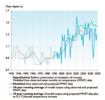
**Fig. 16.28.** Projected thaw depths below the runway at Svalbard Airport (Instanes A. and Mjureke, in press)
