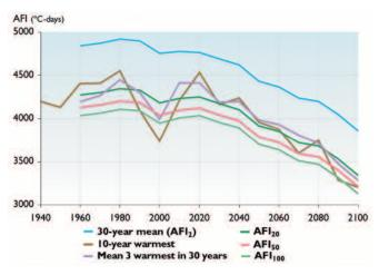
**Fig. 16.26.** Projected air freezing index (AFI) design levels for Kugluktuk (Coppermine), Canada (Instanes A. and Mjureke, 2002b).
