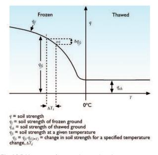
**Fig. 16.5.** Variation in frozen-soil strength with temperature (Ladanyi, 1996).
