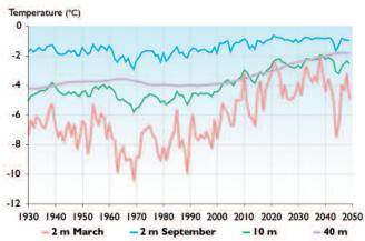
**Fig. 16.29.** Projected ground temperature changes at depths of 2, 10, and 40 m below the Svalbard Airport runway (Instanes A. and Mjureke, in press)
