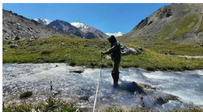
Fig. 46. Measuring stream discharge, northern Tien-Shan (July 2021).
