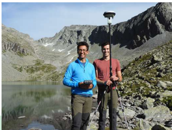
Fig. 2. Satellite-supported surveying of a fixed point in the vicinity of the Arthur-von-Schmidhaus (2281 m asl). View over the Dösen lake to the Dösender rock glacier. Photo: Viktor Kaufmann.
