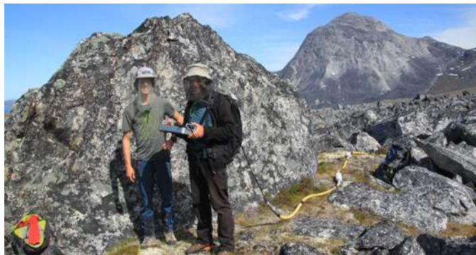
Fig. 3. GPR-campaign at the Bjørneø rock glacier, Greenland using a 100 MHz RTA-antenna. Photo: Andreas Kellerer-Pirklbauer.
