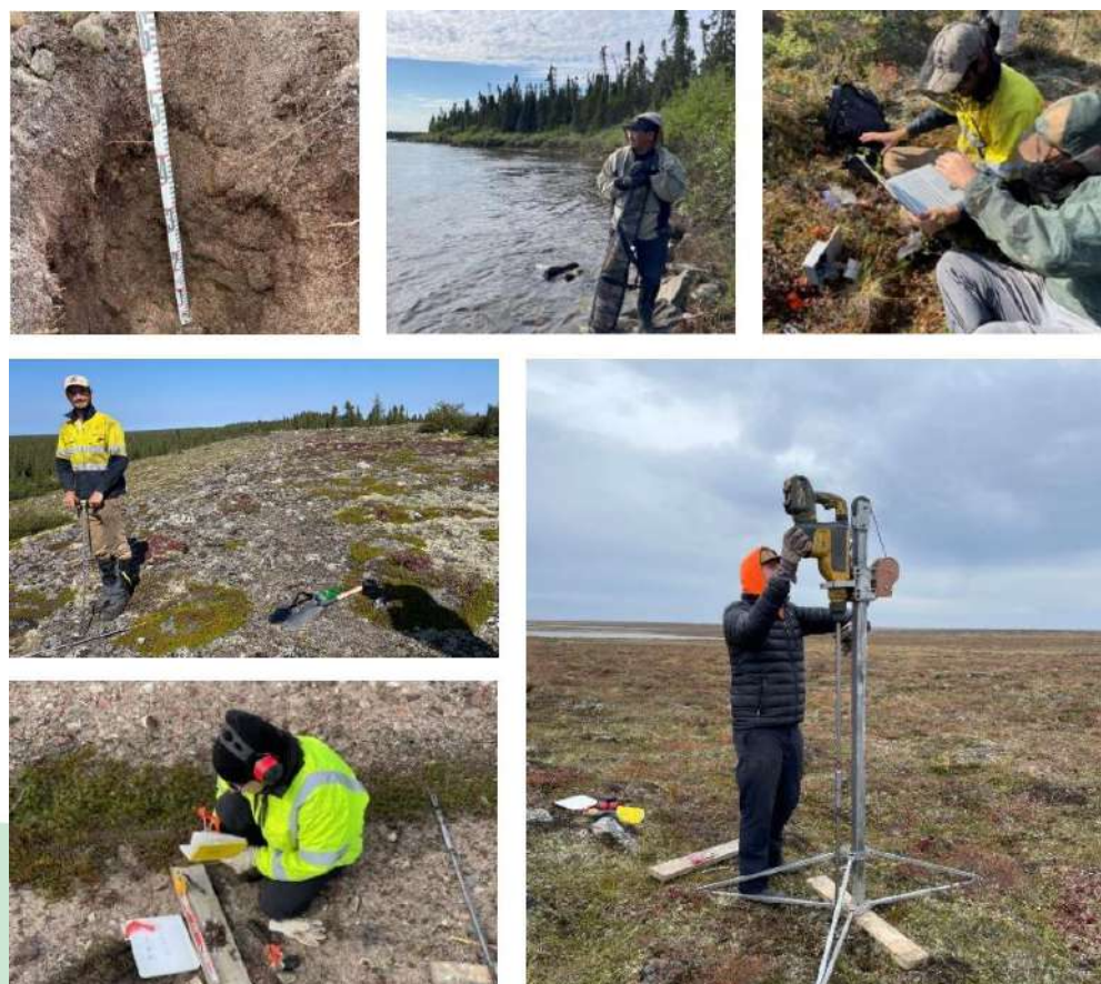
Fig. 10. Clockwise from upper left: soil pit with stadia tape measurements numbered in decimetres, community member ensuring safety from bears, downloading ground temperature data, augering and sampling with the Talon drill, logging frozen drill core, permafrost probing.
