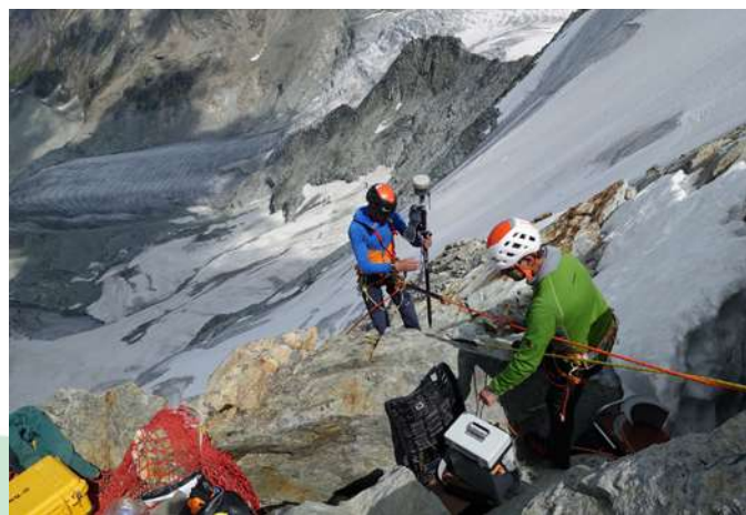
Fig. 56. ERT survey in the north face of the Pointes de Mourti (3563 m asl). Photo: Christophe Lambiel.
