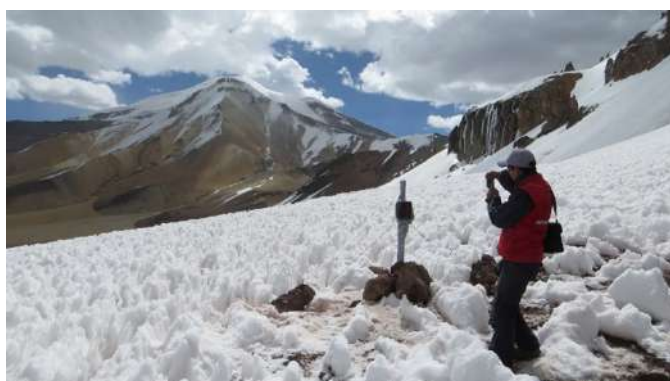
Fig. 54. Air and ground temperature station at 5200 m asl in the Coropuna Volcano.
