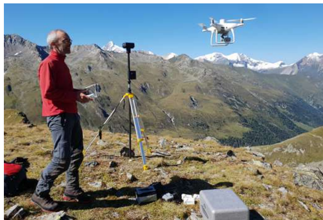
Fig. 4. Launch of a UAV by Gernot Weyss at about 2600 m asl used to survey the rock glacier in the Hinteres Langtalkar, Hohe Tauern Range. Photo: Michael Avian.
