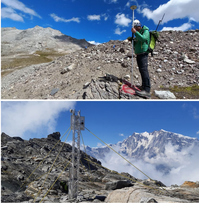
Fig. 29. GNSS-ERT survey at Forneaux (top) and a permafrost monitoring station at Mt. Moro Pass (bottom). Photo: Luca Paro.
