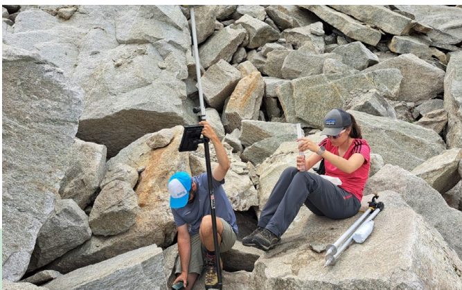
Fig 65. Sampling of the seasonal ground ice at the Monte Prosa rock glacier. Photo: Chantal Del Siro.
