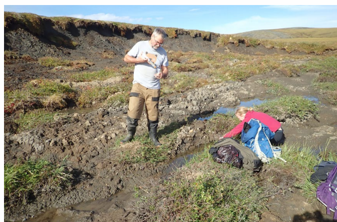
Fig 69. Sampling water and vegetation for sulfur isotope analysis at an RTS, Peel Plateau, NT, Canada (26 August 2022).
