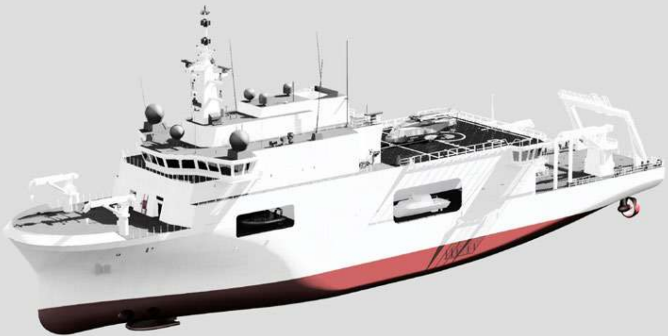
Rendering of the ship Quirinale, the new major hydro-oceanographic vessel of the Italian Navy. The boat, soon to be delivered to the Navy, will have an ICE-7 ice class and an additional notation of Winterization -16 °C, enabling it to operate in polar environments. (credits Hydrographic Institute of the Italian Navy)
