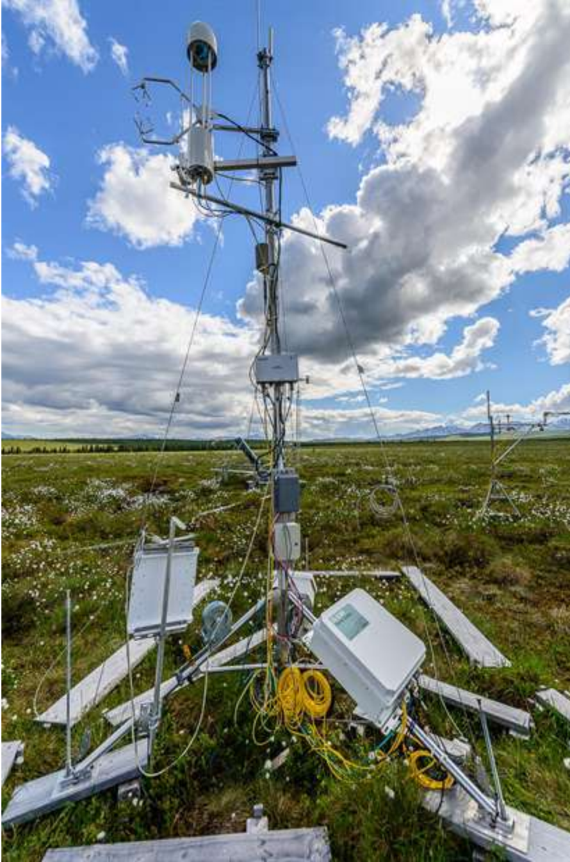
Fig. 2. Eddy covariance tower with micrometeorological sensors and gas analyzers for measuring CO 2 and CH 4 concentrations used to determine the exchange of greenhouse gases between moist acidic tussock tundra and the atmosphere. This tower, located at the Eight Mile Lake research watershed near Denali National Park, Alaska, records aggregated greenhouse gas exchange over 30-minute intervals that can then be combined to determine daily, monthly, seasonal, and annual exchanges of carbon. The tower's sensing footprint is on the scale of tens to hundreds of meters from the tower, depending on windspeed and direction.
